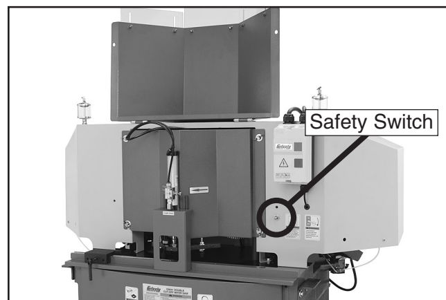
Figure 15. Front guard in the upper position.
